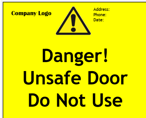
Example unsafe system sign
